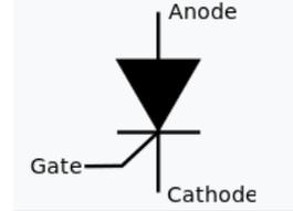
Symbol for an SCR, positive current flows from anode to cathode when the gate is pulsed.
