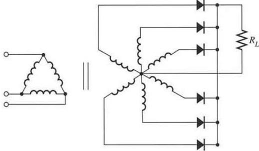
Drawing above shows a typical Delta primary main rectifier transformer with a six-phase star secondary.
