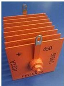
Photo of a multi plate Selenium stack courtesy of Wikipedia
