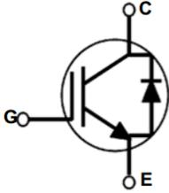
Symbol for an IGBT is courtesy of [completpowerelectronics.com](http://completpowerelectronics.com)
