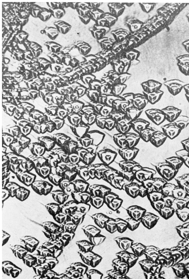
Figure 12 - Etch pits at dislocations in copper. Original magnification 160X (F.W. Young, Jr. 30 ).
