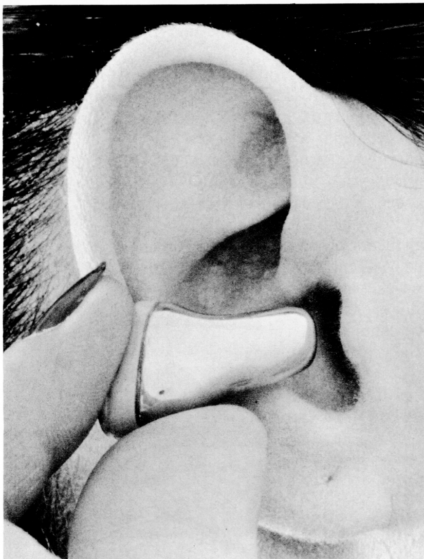
Inside electroformed gold shell are microphone, amplifier, receiver, and other electronics devices covered with faceplate.
