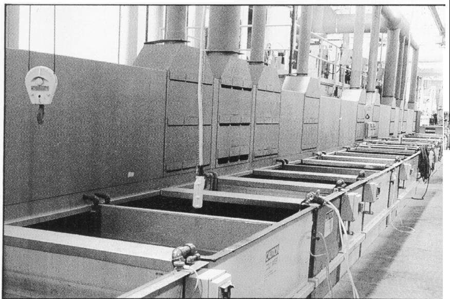
Pratt and Whitney's North Haven facility has a new nickel plating and titanium cleaning line.
