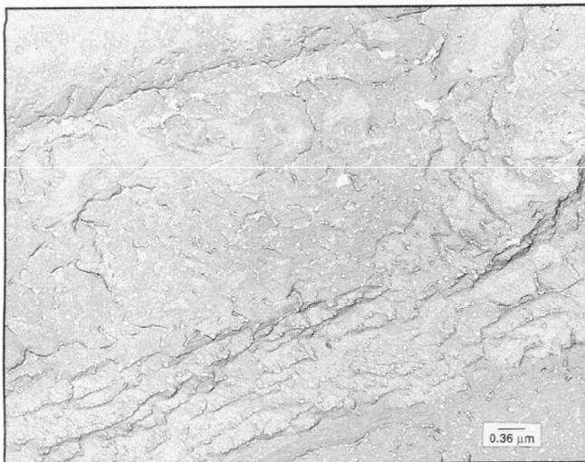
Fig. 7—TEM of high-phosphorus EN coating.
