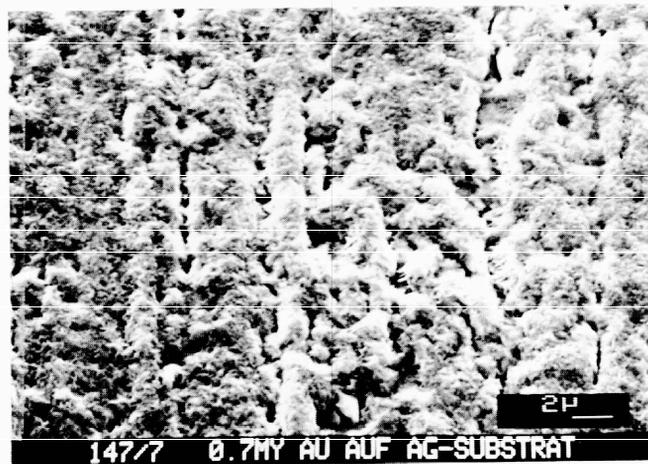
Fig. 11—SEM of gold deposited from Bath ELI (15 g/L KCN, 80° C) on silver.
