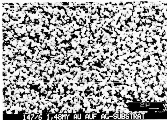
Fig. 12—SEM of gold deposited from Bath EL1 (10 g/L KCN, 80° C) on silver.
