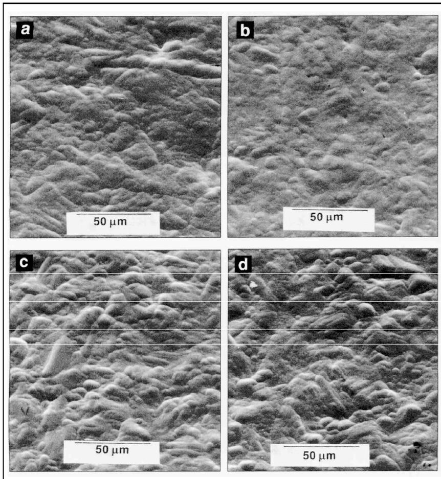
Fig. 6-Scanning electron micrographs of electroless nickel-phosphorus coatings under different magnetic stirring [clockwise/counter-clockwise (A/D)] rates; (a) 250 rpm, (b) 300 rpm (c) 350 rpm (d) 400 rpm. Operating conditions: pH 4.5, 85 °C; plating time, two hr.
