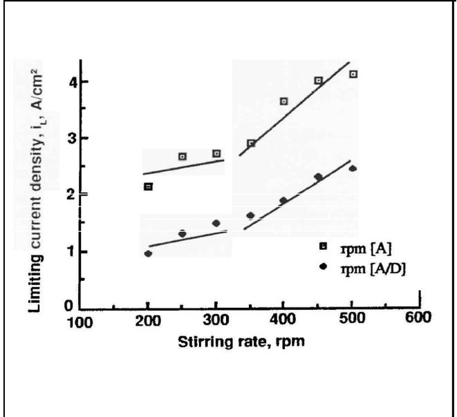
Fig. 9—Limiting current vs. magnetic stirring clockwise [A] and counter-clockwise [D], using an acid copper electrolyte;  $i_L$  obtained at  $E = -0.75$  V.
