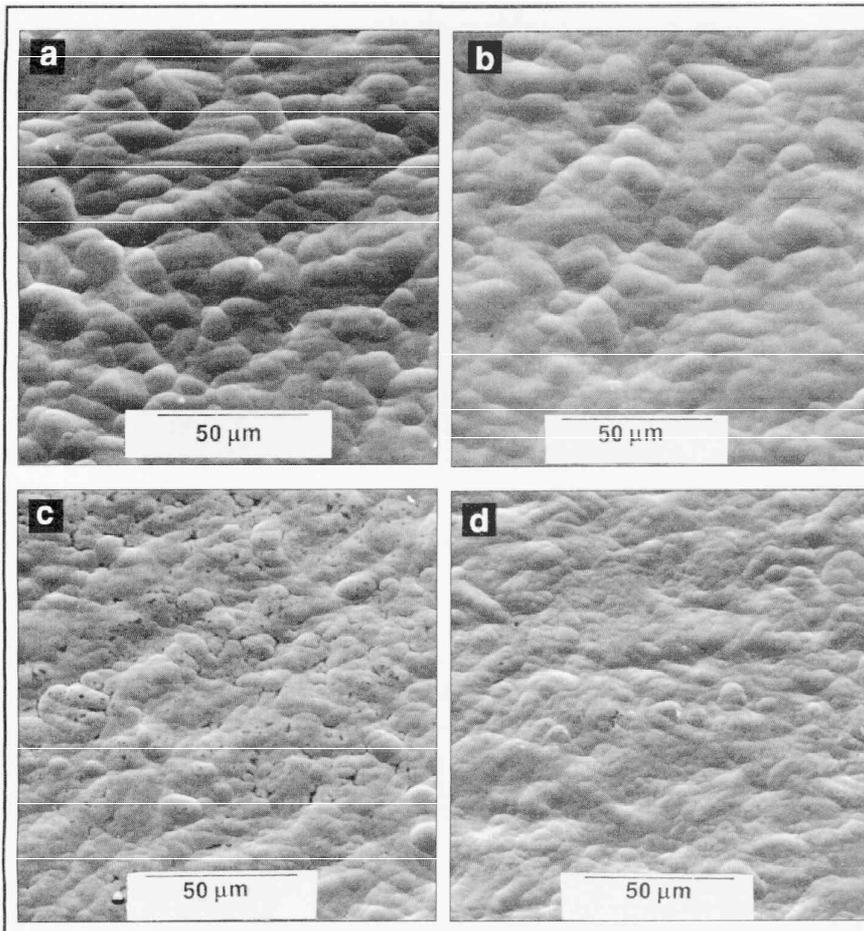
Fig. 5-Scanning electron micrographs of electroless nickel-phosphorus coatings under different magnetic stirring [clockwise] rates; (a) 250 rpm, (b) 300 rpm, (c) 350 rpm, (d) 400 rpm. Operating conditions: pH 4.5, 85 °C; plating time, two hr.
