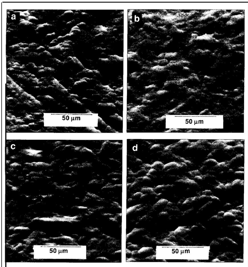
Fig. 4—Scanning electron micrographs of electroless nickel-phosphorus coatings under natural convection and different aeration rates; (a) 0 rpm, (b) 3.0 L/min, (c) 3.5 L/min, (d) 4.5 L/min, Operating conditions.. pH 4.5, 85°C; plating time, two hr.
