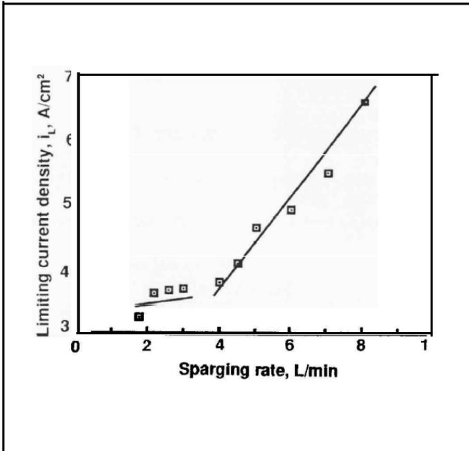
Fig. 10—Limiting current vs. different sparging agitation rates, using an acid copper electrolyte;  $i_L$  obtained at  $E = -0.75$  V.
