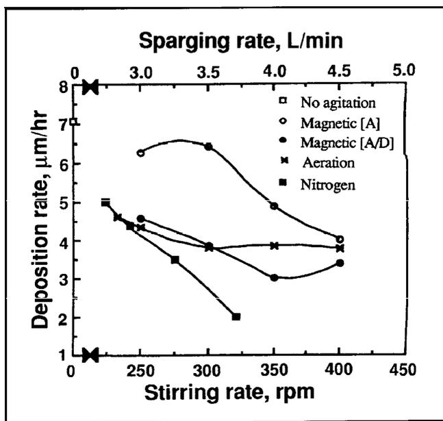
Fig. 2—Effect of different types and rates of agitation on deposition rate, using the electroless Ni-P solution operated at-pH 4.5 and 850 C
