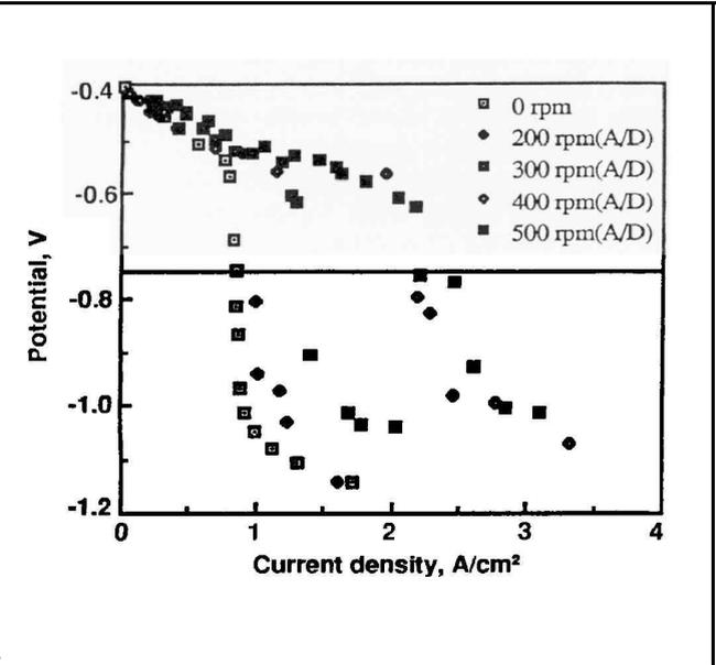
Fig. 8—Polarization curves obtained using an acid copper sulfate electrolyte under different magnetic stirring (clockwise/counter-clockwise) rates.
