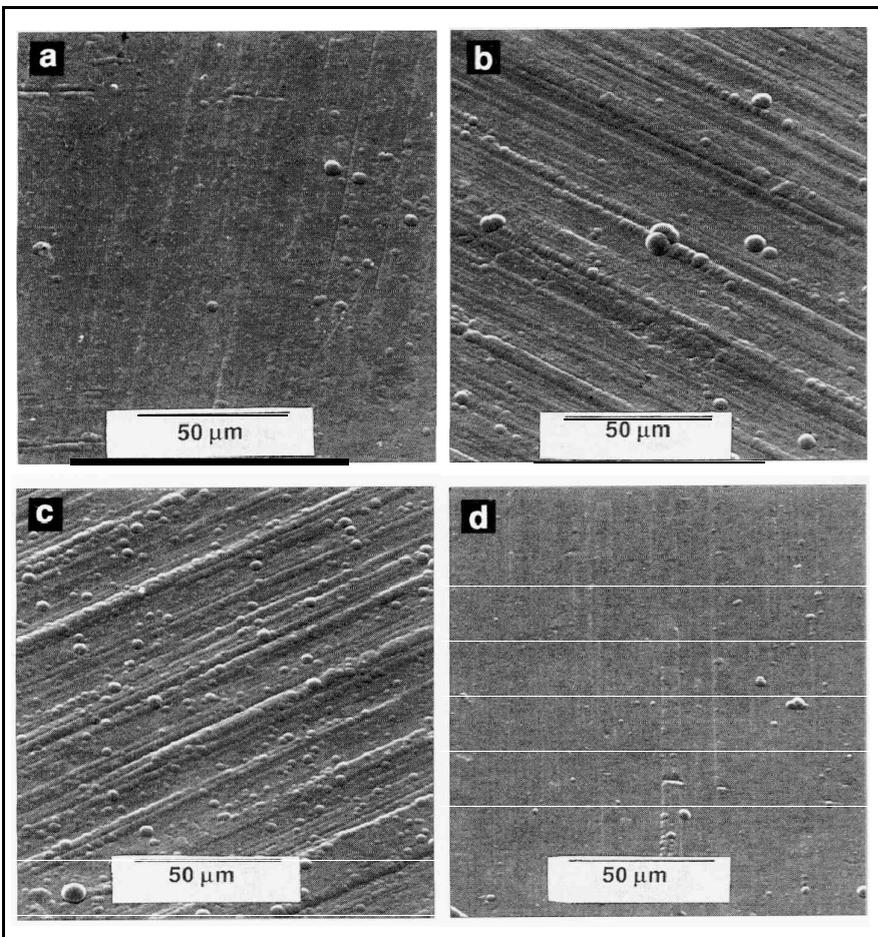
Fig. 7—Scanning electron micrographs of electroless nickel-phosphorus coatings under different nitrogen sparging rates; (a) 2.69 L/min, (b) 2.92 L/min, (c) 3.00 L/min, (d) 3.85 L/min. Operating conditions: pH 4.5, 85°C; plating time, one hr.
