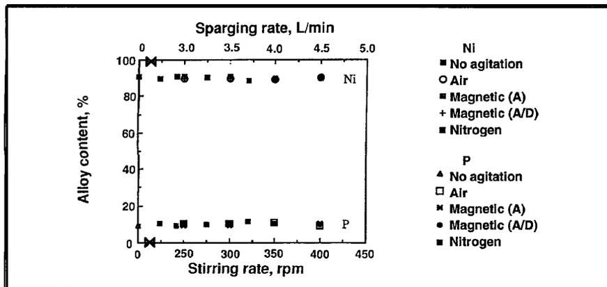
Fig. 3—Percentage of nickel and phosphorus in the deposited coatings under different agitation types and rates and their comparison to no agitation. A—magnetic stirring clockwise; D—magnetic stirring counter-clock wise.
