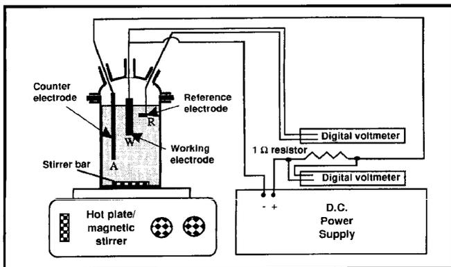
Fig. 1—Experimental arrangement used for polarization studies.
