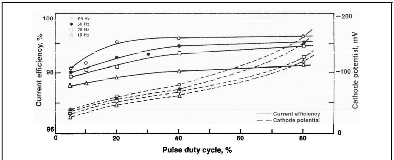
Fig. 5—Effect of pulse duty cycle on cathode current efficiency and cathode potentials of copper deposition at 2.5 A/dm<sup>2</sup> average current density.
