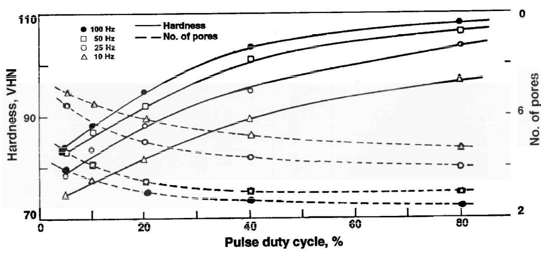
Fig. 6—Effect of pulse duty cycle on hardness and porosity of copper deposits at 2.5 A/dm<sup>2</sup> average current density.
