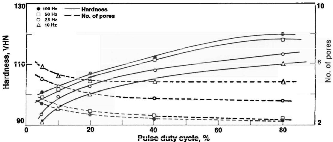
Fig. 10—Effect of pulse duty cycle on hardness and porosity of copper electrodeposited at 7.5 A/dm<sup>2</sup> average current density.
