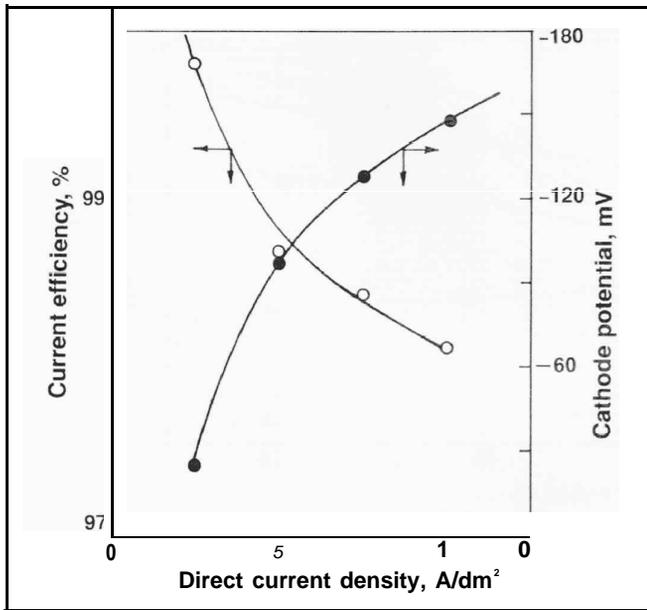
Fig. 3—Effect of current density on current efficiency and cathode potential during DC copper deposition (DC).
