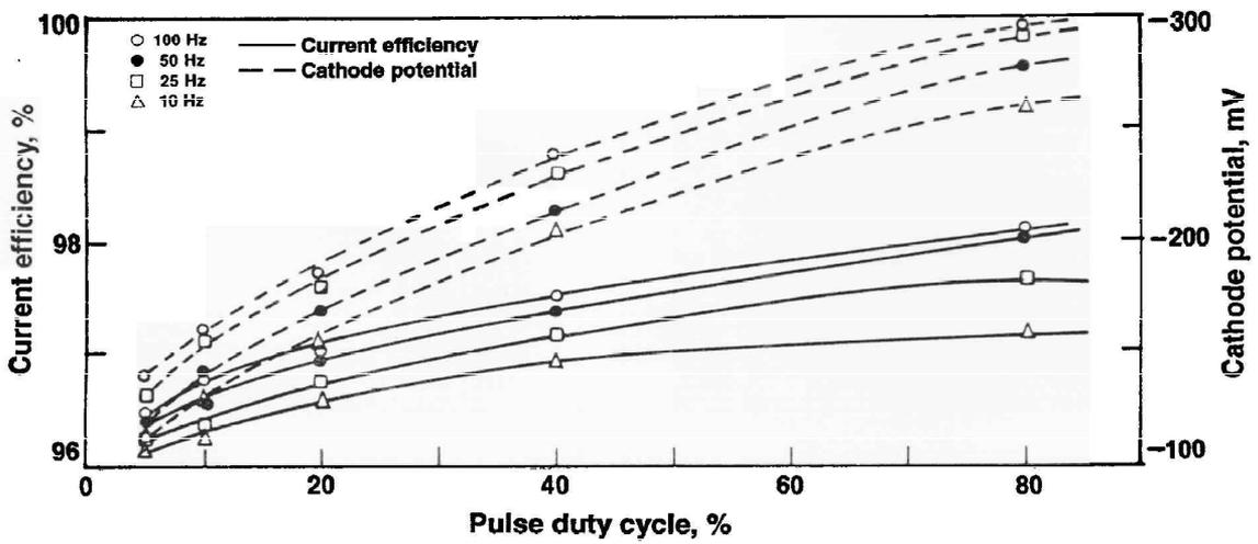
Fig. 9—Effect of pulse duty cycle on cathode current efficiency and cathode potentials of copper deposition at 7.5 A/dm<sup>2</sup> average current density.
