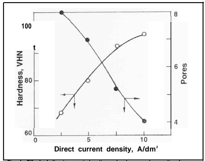
Fig. 4—Effect of direct current density on hardness and porosity of copper deposits.
