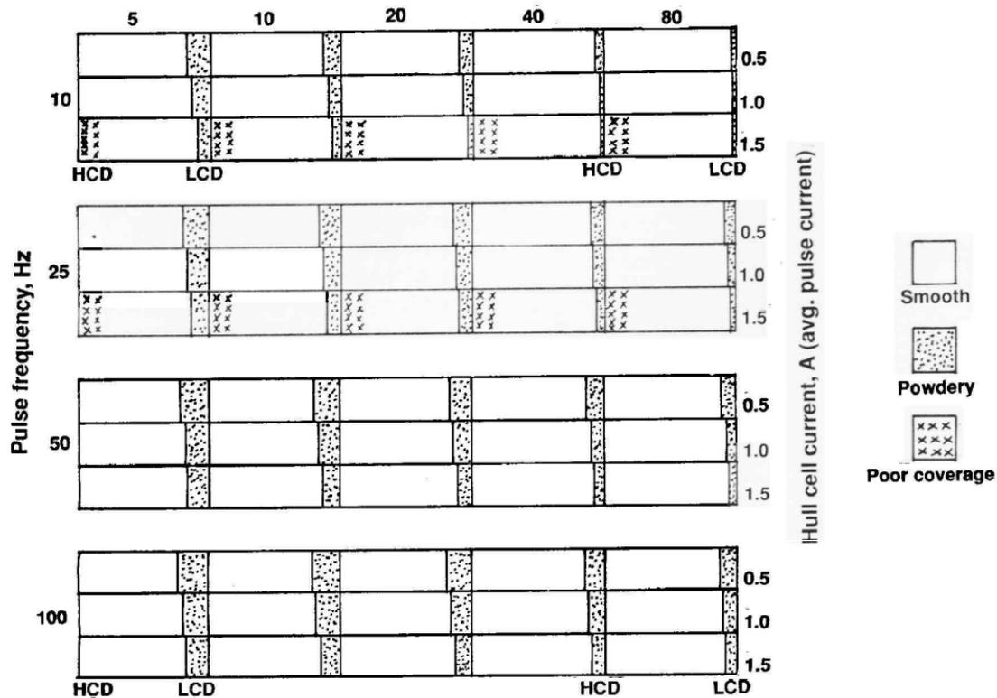
Fig. 2—Hull Cell panels plated under different pulse conditions.
