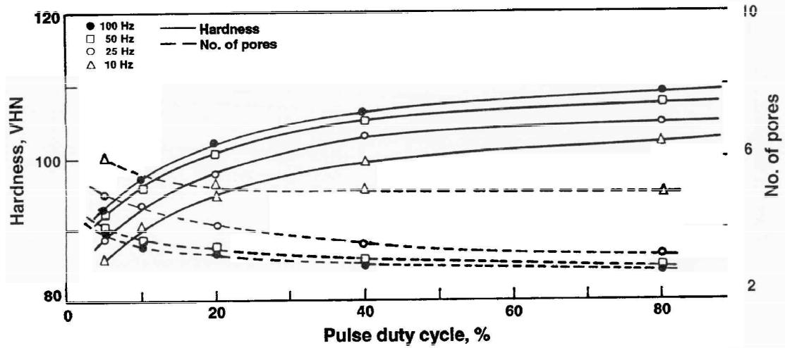
Fig. 8—Effect of pulse duty cycles on hardness and porosity of copper deposits at 5 A/dm<sup>2</sup> average current density.
