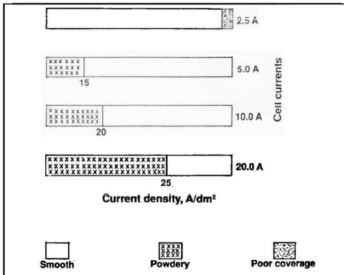
Fig. 1—Hull Cell panels plated with copper at different cell currents (DC).
