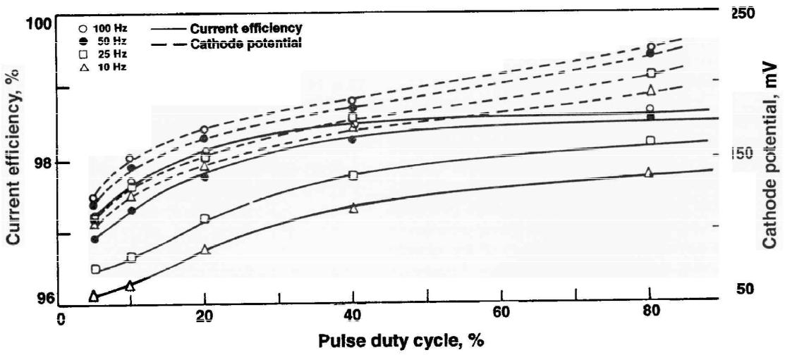
Fig. 7—Effect of pulse duty cycle on cathode current efficiency and cathode potentials of copper deposition at 5 A/dm<sup>2</sup> average current density.
