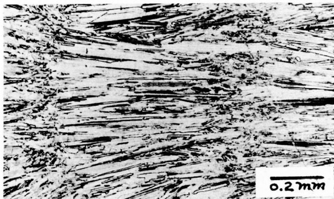
Fig. 16—Optical micrograph of cross section of copper deposit.
