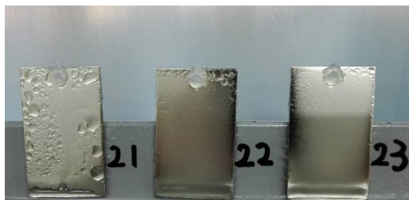
Figure 5 - 6-micron Hybrid \text{Al}_2\text{O}_3 with semi-bright and bright nickel after 102 hr of salt spray testing.
