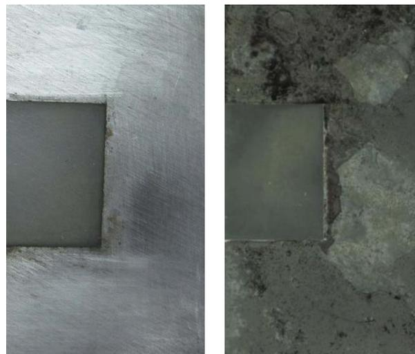
Figure 8 - Test of Co-Cr<sub>3</sub>C<sub>2</sub> for oxidation resistance: (L) as-plated; (R) after 800°C for 30 hr in air.
