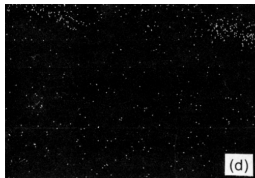
Figure 10 - (a) SEM electron image of section through Ni/Au conductor reflow-soldered (63% Sn/37% Pb) interface following aging at 135°C for 1200 hr; scale marker = 5 \mu m; (b) Ni X-ray image for "a"; (c) Sn X-ray image for "a"; (d) Pb X-ray image for "a".
