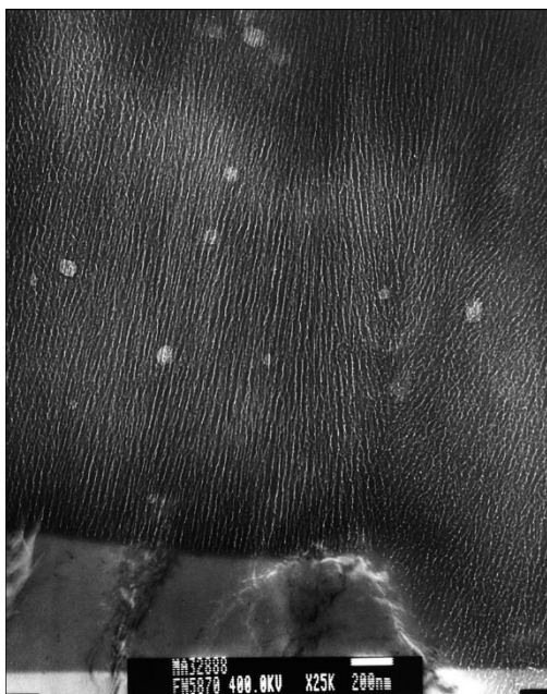
Figure 4 - Representative TEM micrograph of a Type II anodic oxide finish.
