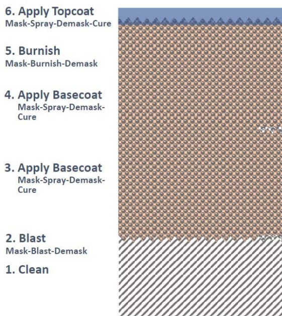
Figure 2 – Schematic of the chromate/phosphate system.
