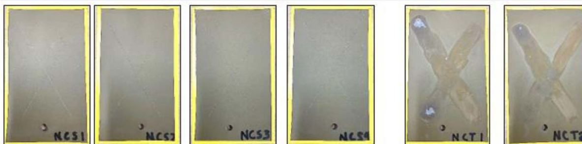
Figure 6 – Coated steel panels after 50-day U.S. Navy cyclic test. The first pair of panels in each row were coated with sacrificial basecoat alone (with no seal coat) and scribed, the second pair of panels were coated with sacrificial base coat and seal coat and then scribed, the third pair of panels were coated with sacrificial base coat, sealed, scribed and then touched up. Performance of Alseal 5KGT (lower row) was equal to or better than that of the legacy system (top row)
