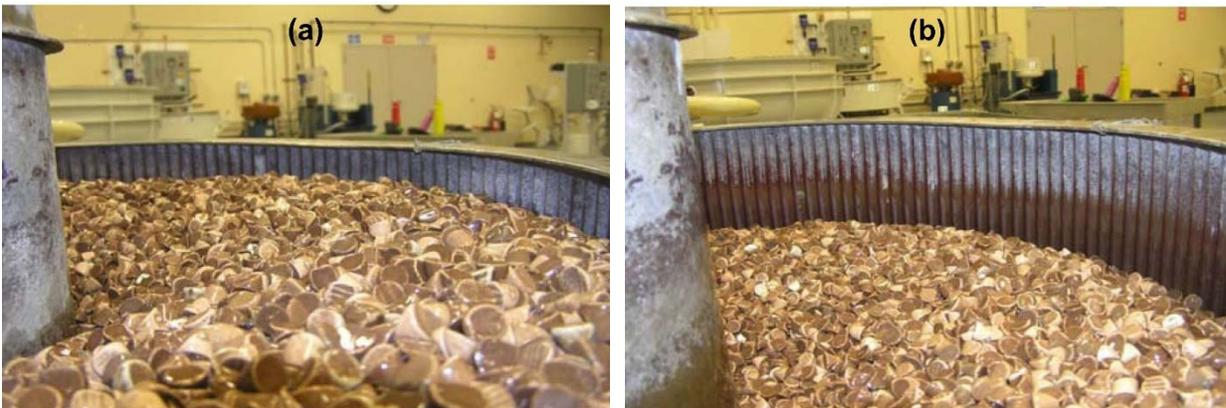
Figure 2 - Image of a vibratory bowl (a) with the proper depth of media present in the bowl channel and (b) where the media depth is too low, caused by attrition.<sup>6</sup>
