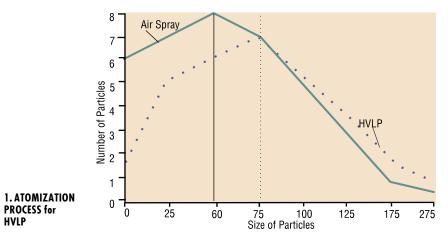
The more material you use, the greater the output of VOCs to the atmosphere. Increasing transfer efficiency can decrease the overall quantity of material used and thus decrease the total VOCs emitted.
