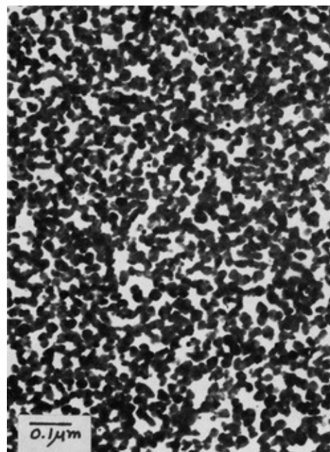
Figure 2 - Transmission electron micrograph of non-epitaxial nuclei (gold).
