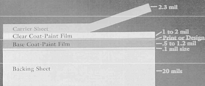
Cross Section of paint film laminate
