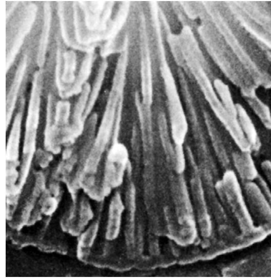
Figure 4 - Higher-magnification view of Fig. 3 shows pore branching and inclination of divergent pores.
