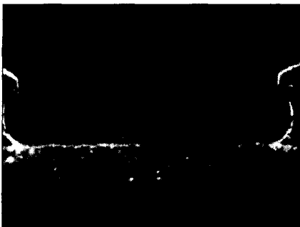
Figure 11. Microscopic metal track between SMT pads.
