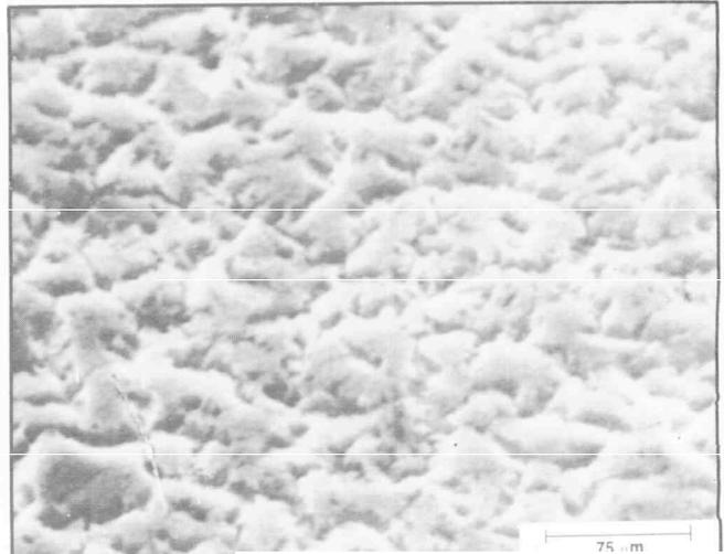
Fig. 10—SEM photograph of zinc with an iridescent chromate coating. Magnification: 1 cm = 25 μm.
