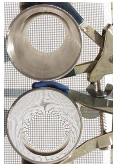
Figure 7 - 316SS tube surface before (top) and after (bottom) sequenced pulse reverse electropolishing in a NaCl-NaNO<sub>3</sub> electrolyte.
