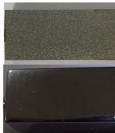
Figure 10 - Electropolished powder bed additively manufactured Ti-6Al-4V.
