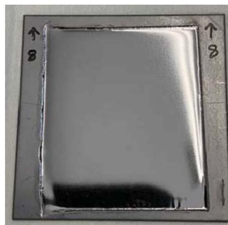
Figure 9 - Electropolished 2" x 2" tantalum coupon. Edge shows surface prior to polishing.
