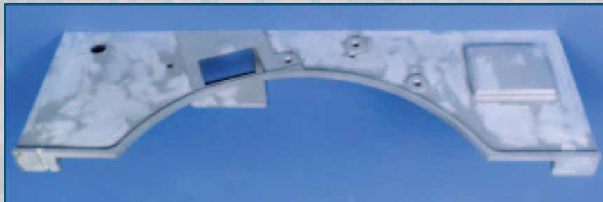
The material used to fill holes in the castings can withstand temperatures of more than 1,000 °F.
