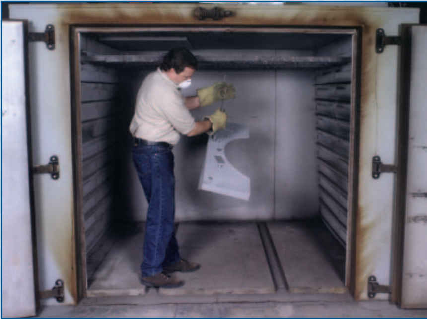
The powder coated aprons are baked in a batch oven at 420 °F for about 15 min to melt the nylon coating, cooled, coated and baked a second time.
