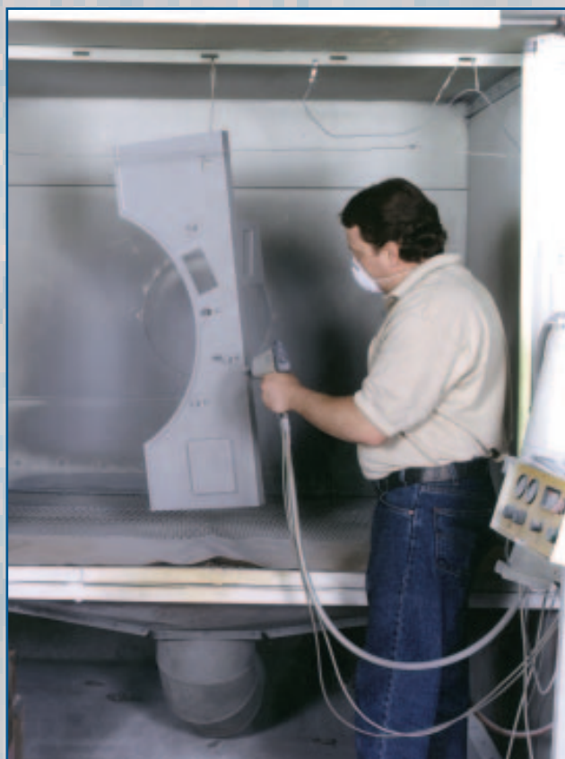
Spray booths are used to apply the electrostatic powder coating. The technique provides 90 percent transfer efficiency, substantially reducing waste disposal costs.
