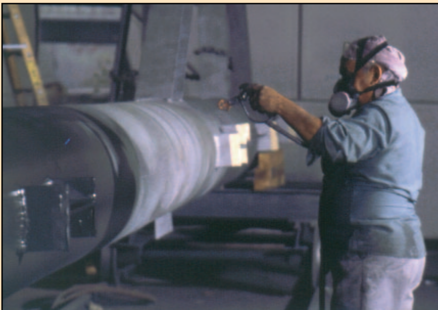
By eliminating the need for lifts or scaffolding, coatings can be applied in a fraction of the time compared to conventional on-site application.
