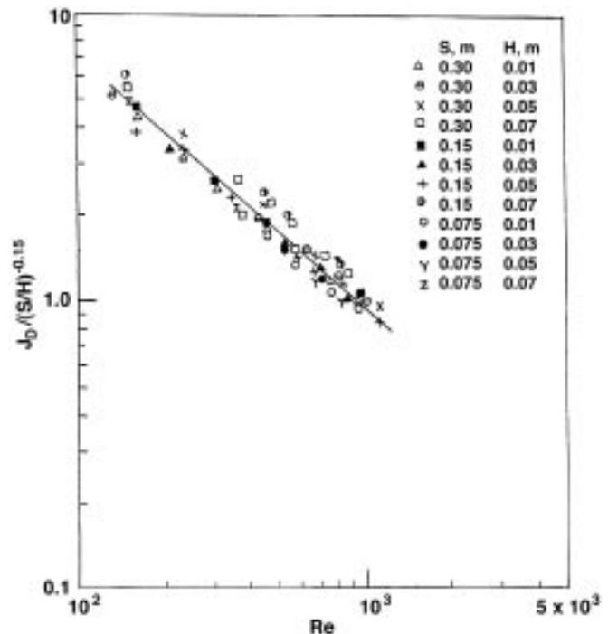
Fig. 10—Correlation plot of average coefficient of columns 2 and 3 in accordance with Eq. (4).
