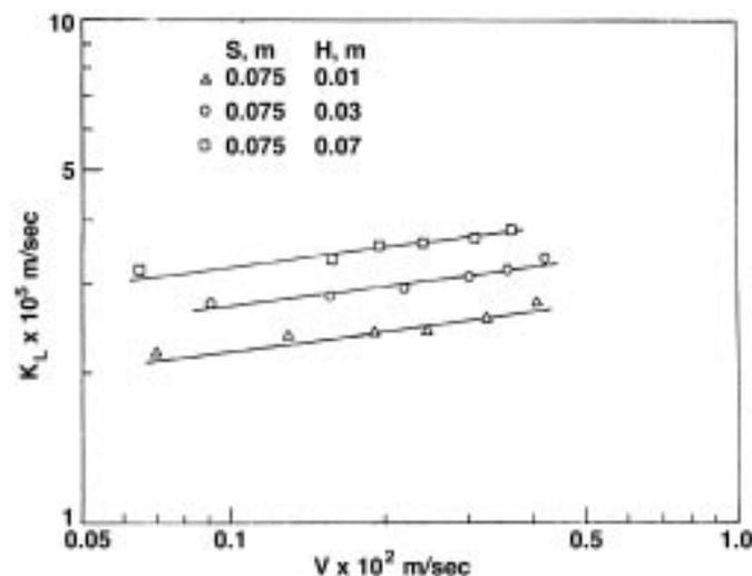
Fig. 4—Effect of propromter height on overall coefficients at  $S = 0.075$  m.
