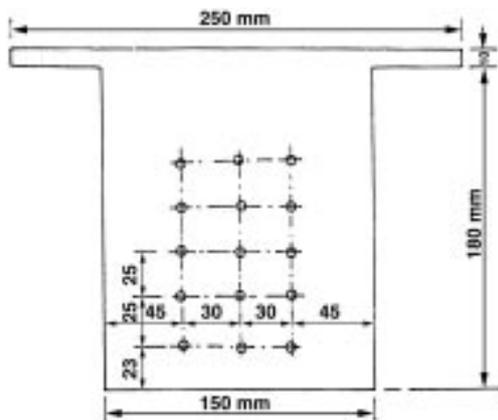
Fig. 1—Cathode support plate (dimensions in mm).
