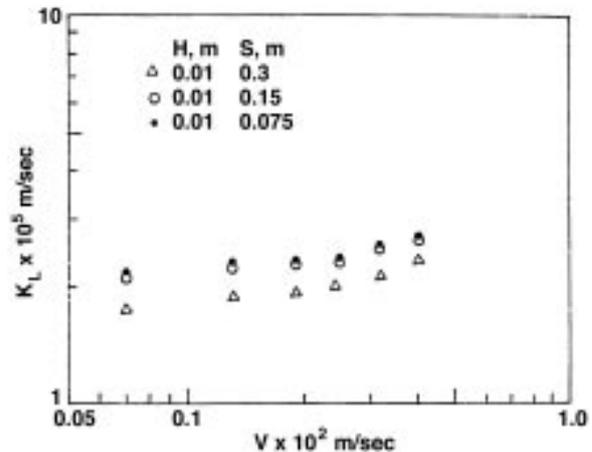
Fig. 8—Effect of promoter spacing on average coefficient of columns 2 and 3.
