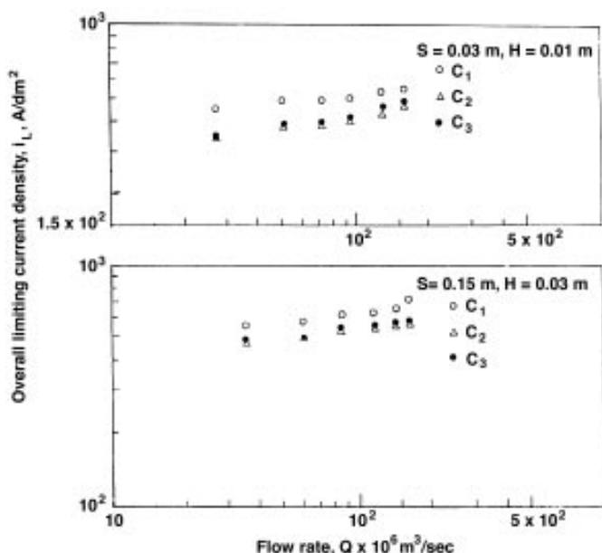
Fig. 3—Plot of overall limiting current density vs. flow rate at columns 1, 2 and 3 of CSP.
