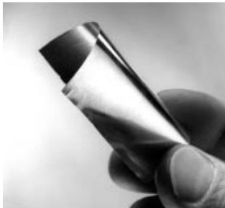
Fig. 11—Electroformed 80/20 Pd-Co @ 20-40 wt pct Co.
