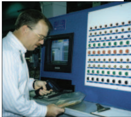
Brian Day, CEF, senior processing engineer at Kaynar, shows off some of the fasteners in bins in the nut staging area. Some of the finishes visible here include silver and cadmium plating, and chromate conversion coating.
