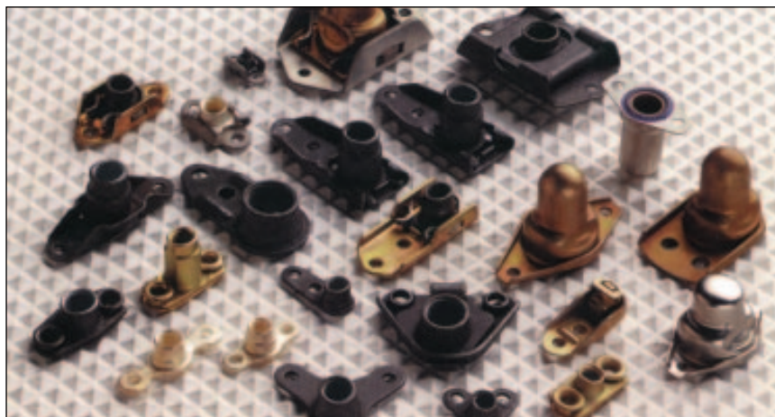
(Top left) Gang channels—Produced in straight or radiused versions, these assemblies are for applications that require multiple, equally spaced anchor-type nuts. Gang channels enable rapid assembly and disassembly of structure sections. Typical applications include opening around aircraft access doors and leading edges. (Top right) Barrel nuts—High-strength, self-locking nuts for use in locations where wrenching space is not available. Typical applications include the assembly of aircraft wings and tail attachments. Made of alloy steel, corrosion-resistant steel and Inconel, finishes include Cd plating and solid film lubricants. (Bottom) Anchor nuts—Especially useful in blind locations or where an attached nut facilitates maintenance. The nut mounting lugs may be riveted, welded or screwed to the structure. They insure positive positioning of the mating bolt and are self-wrenching. Special nuts, such as self-sealing domes, prevent fuel leaks.
