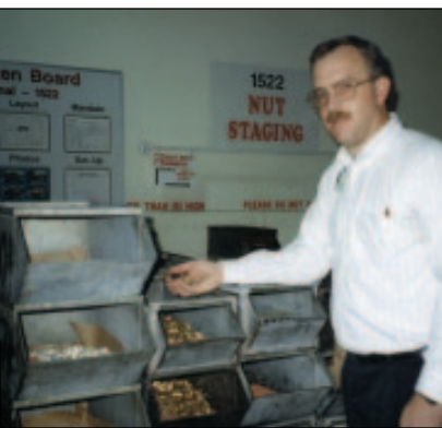
Brian Day, CEF, senior processing engineer at Kaynar, shows off some of the fasteners in bins in the nut staging area. Some of the finishes visible here include silver and cadmium plating, and chromate conversion coating.
