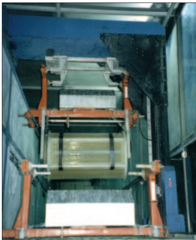
Plating lines are fully enclosed to keep out contaminants and make it easier to contain and exhaust fumes.
