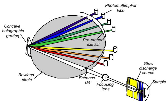
Fig. 2 - The Grimm-type GD-OES source and the UV-VIS polychromator, as the commercial LECO SDP-750 spectrometer
