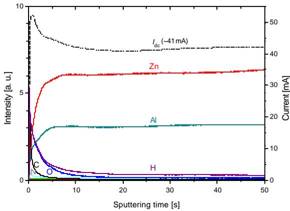
Fig. 5 - Depth profiling of a bulk Zn-sample
