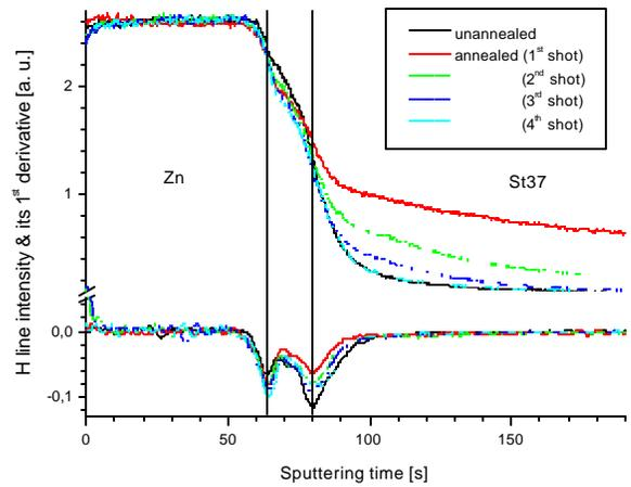
Fig. 7 – Depth profiles of electrolytically deposited Zn layer: (i) unannealed (black curve) and (ii) annealed (red curve) 24 h, 220°C in Argon.
