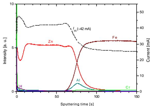
Fig. 4 - Depth profiling of a Zinc layer deposited by hot dip galvanising
