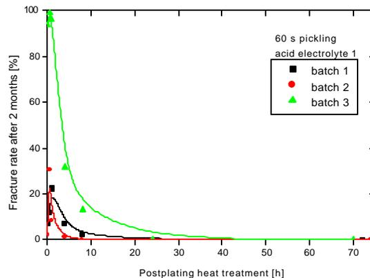
Fig. 1- Fracture rate of Zn-plated fuse holder rings with respect to the annealing time at 220°C
