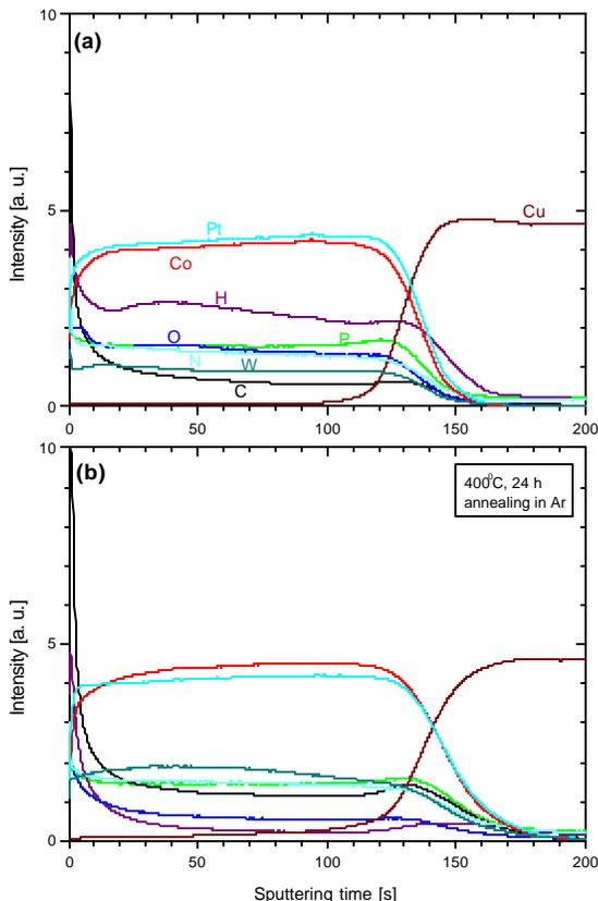
Fig. 6 - Depth profiling of an electrolytically deposited CoPt-layer as plated (a) and after annealing (b)
