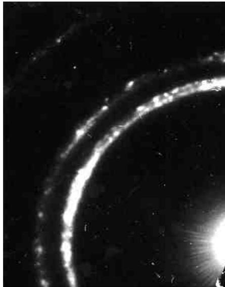
*Figure 5* Enlarged Image of Electron Diffraction Pattern of Chromium Replacement Alloy Coating
