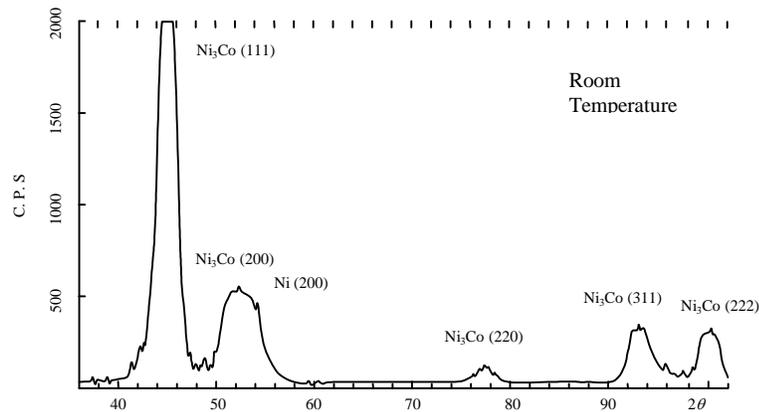
Figure 1 X-ray Diffraction Pattern of Chromium Replacement Alloy Coating at Room Temperature
