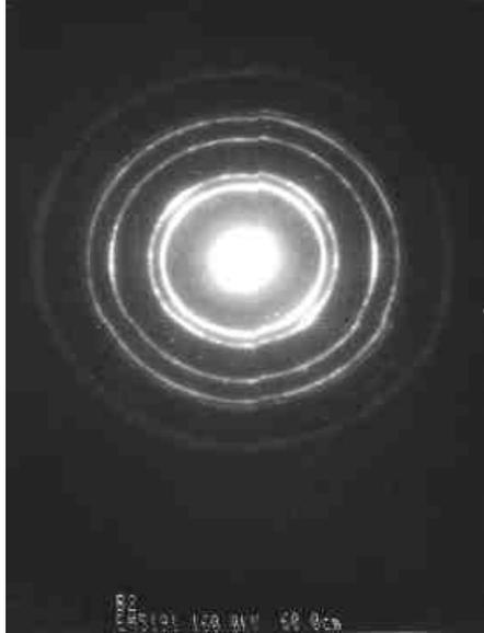
*Figure 3* Electron Diffraction Pattern of Chromium Replacement Alloy Coating
