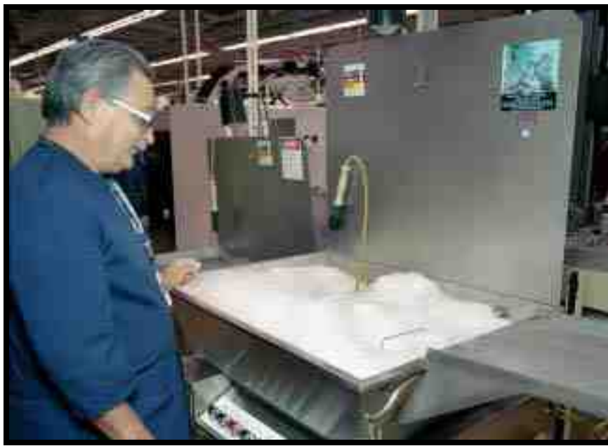
Figure 10. Ultrasonic cleaning system for precision hardware.
