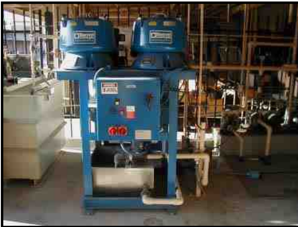
Figure 7. Centrifuge based recycling system in vibratory deburr area.
