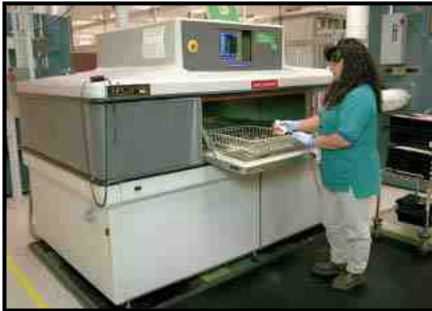
Figure 9. Wash unit for cleaning circuit cards prior to parylene coating.
