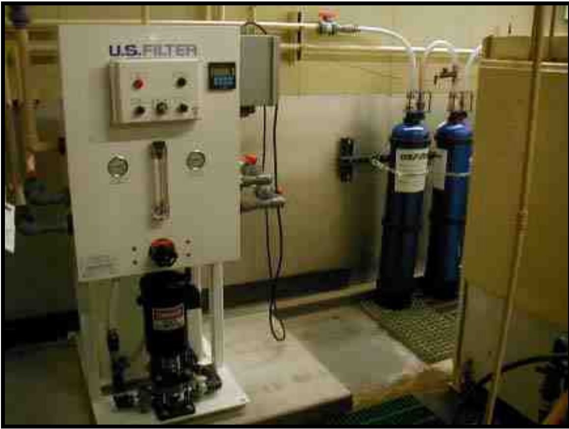
Figure 5. Rinsewater recycler at electrochemical deburr station.
