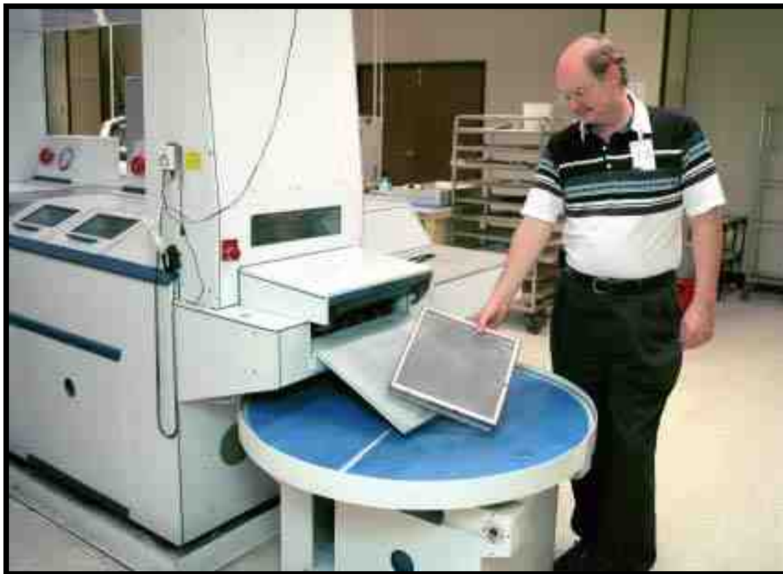
Figure 8. Fully aqueous wash system for removal of HF1189 flux from circuit cards.
