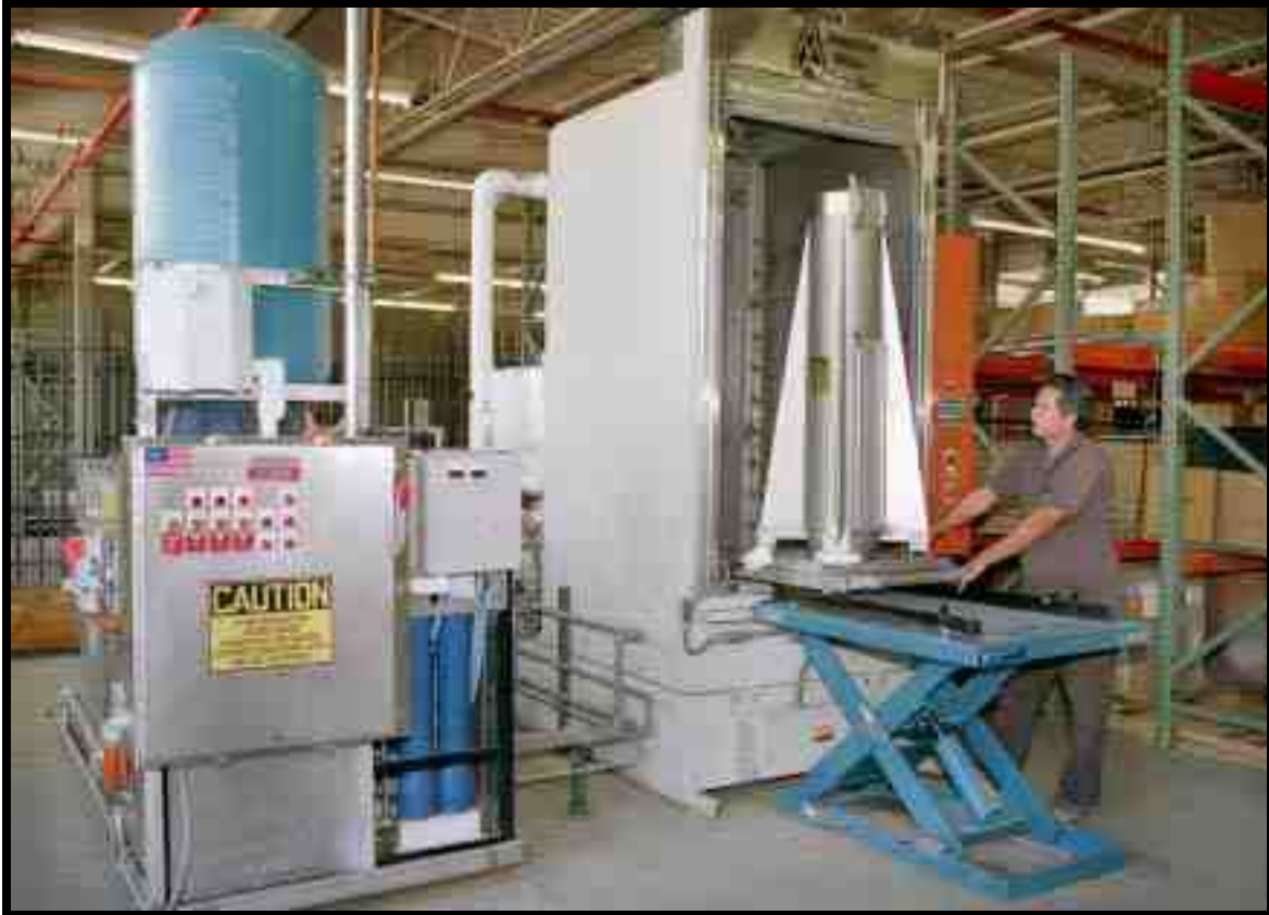
Figure 2. Aqueous cleaner recycling system (left) integrated with wash unit (right).
