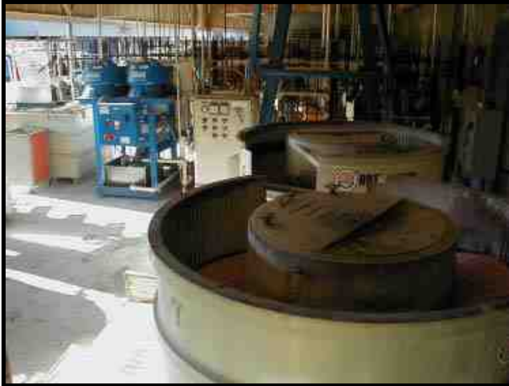
Figure 6. Vibratory Deburr Units for removing burrs from machined hardware.
