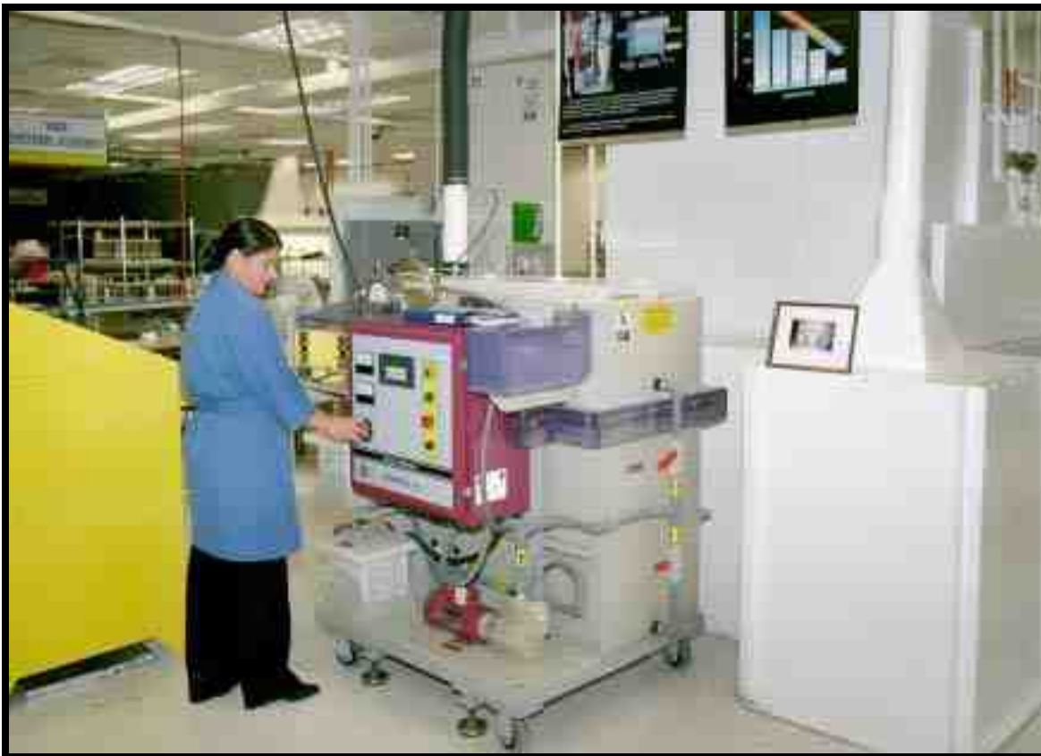
Figure 3. Electroflotation unit recycles paint booth waters from lacquer spray operation.
