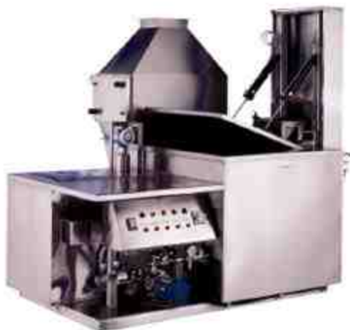
Figure 4. – A collector with condenser for plating waxes with melting points above 85 C (185 F).
