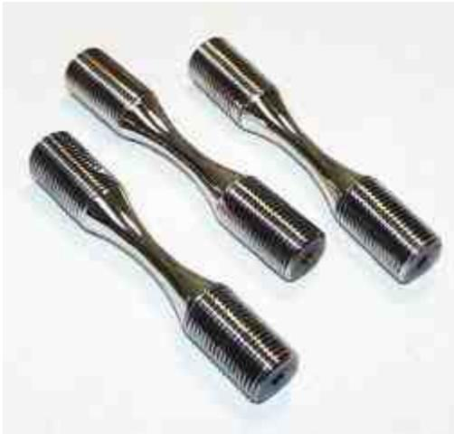
**Figure 6** Photograph of the 43040 wear samples coated with nanocrystalline Co 2-3wt% P.
