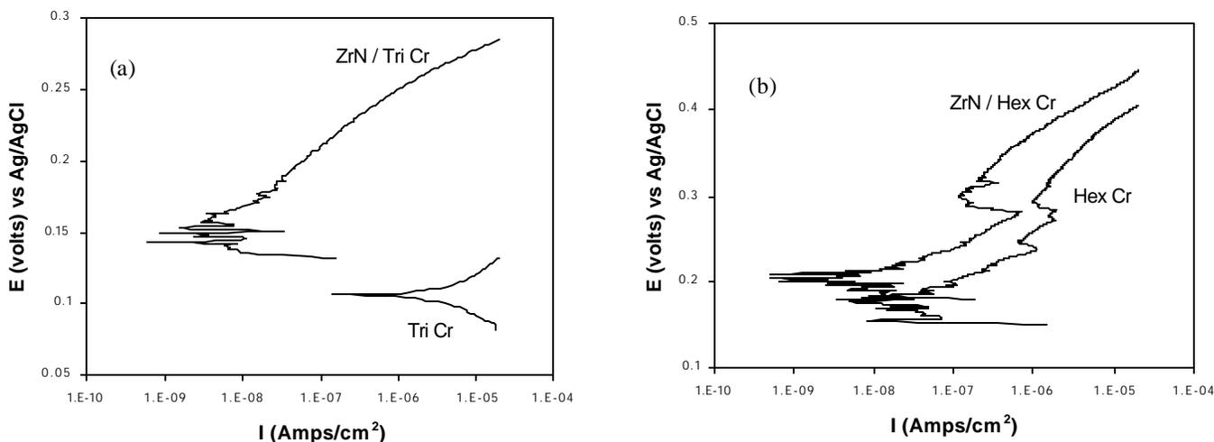
**Figure 2.** Potentiodynamic responses for as-received Cr/Ni/Brass samples versus ZrN coated Cr/Ni/Brass for (a) trivalent Cr and (b) hexavalent Cr.
