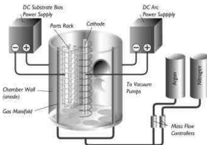
Figure 1. Schematic of LTAVD chamber used for ZrN deposition.
