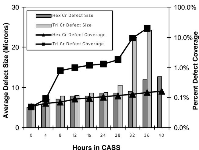
Figure 4. Plot of CASS results on as-received chromium plating throughout 40 hours of testing.
