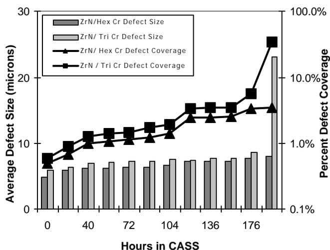
Figure 4. Plot of CASS results on ZrN coated chromium plating throughout 196 hours of testing.
