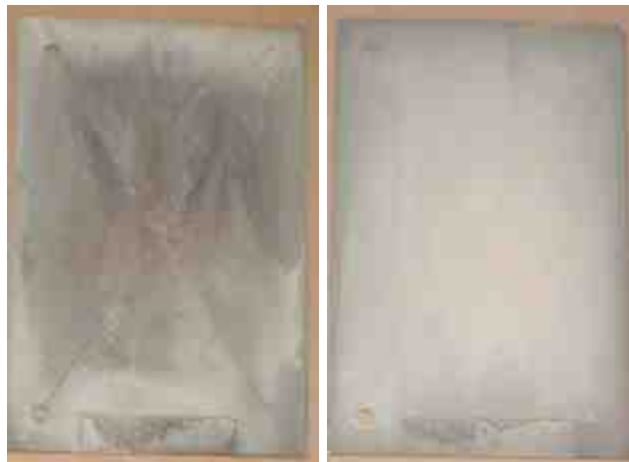
Figure 11: Cadmium with chromate (R) and TCP (L) after 1000 hours of ASTM B 117 salt fog
