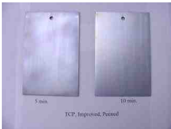
Figure 14: Modified IVD Al, peened, with 5 and 10 min TCP
