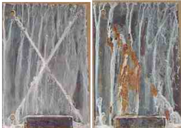
Figure 9: Dipsol Gumm Zn-Ni with chromate (R) and TCP (L) after 1000 hours of ASTM B 117 salt fog
