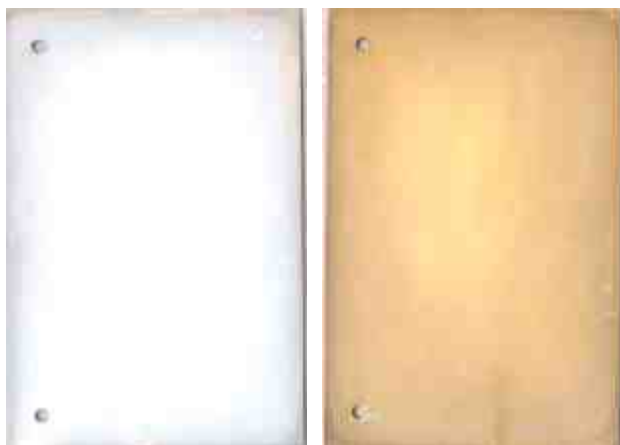
Figure 5: Cadmium with chromate (R) and TCP (L)
