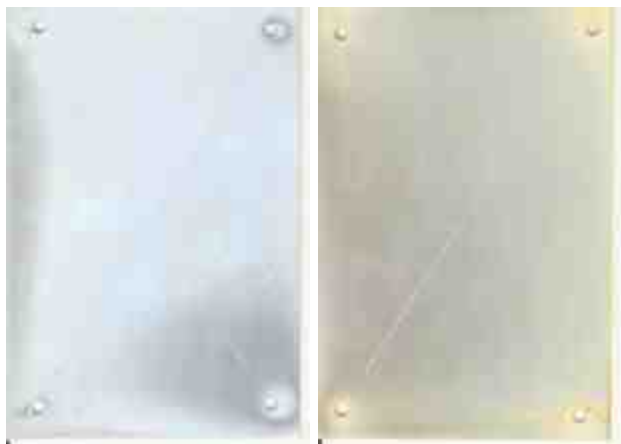
Figure 1: Alumiplate with chromate (R) and TCP (L)
