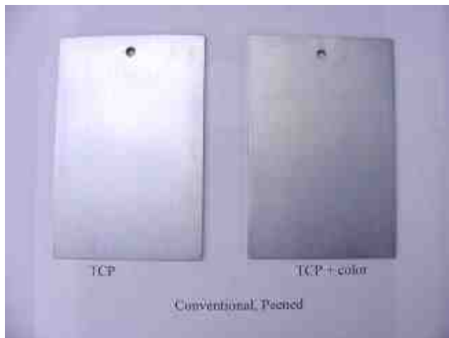
Figure 15: Conventional IVD Al, peened, comparing TCP to TCP with color change
