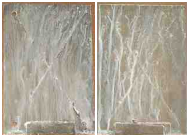
Figure 10: Tin-Zinc with chromate (R) and TCP (L) after 1000 hours of ASTM B 117 salt fog
