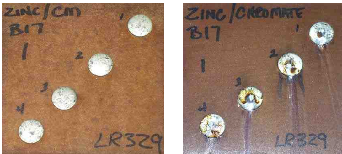
Figure 2: ASTM B117 Salt Spray Performance of “bucked” rivets at 1000 hours using coating systems with and without the mineral coating. Left: Zinc plate with mineral coating topcoated with chromate containing heat-cured epoxy. Right: Zinc plate with yellow chromate (Cr(VI)) topcoated with same chromate-containing heat-cured epoxy.
