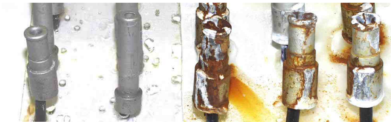
Figure 1: ASTM B117 Salt Spray Performance of end-fitting fasteners at 3000 hours using coating systems on left: Zinc plate with the mineral coating topcoated with chromate-containing heat-cured epoxy, and on right: Zinc plate with yellow chromate (Cr(VI)) topcoated with same chromate-containing heat-cured epoxy.
