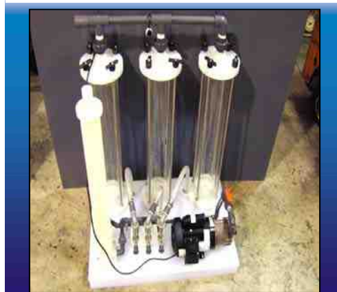
Figure 3, Typical design for an ion exchange and filter system used with trivalent chromium
