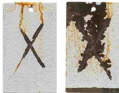
Figure 10, Powered coated panels scribed and NSS tested for 168 hours - Left panel new system pretreatment - Right panel conventional phosphate
