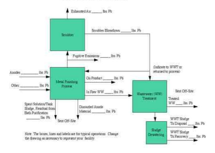
Figure 1. Material Balance for Lead
