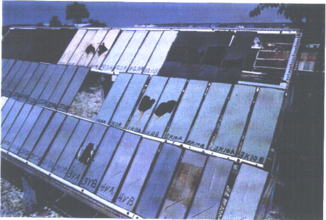
FIGURE 12: PANELS EXPOSED TO 45° SOUTH ON MARINE TEST FENCE
