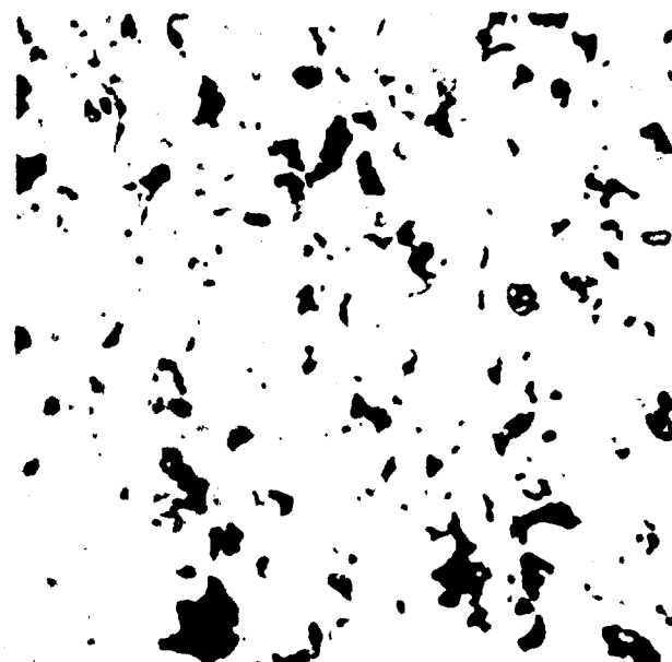
Spec. 244, (C-MCC 50-20) (Sintered), after 1 hr screening at T_h = 1200^\circ\text{C} , and 1 hr at 1300^\circ\text{C} in helium, unetched, 600X
