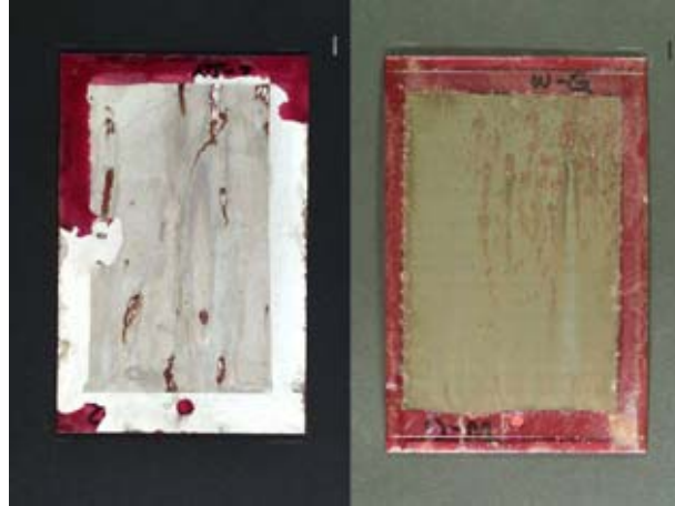
Figure 16. Comparison of 0.005”-Thick Electrodeposited Hard Nickel and HVOF WC/17Co After 20 Days of Exposure in the B117 Salt-Fog Cabinet.
