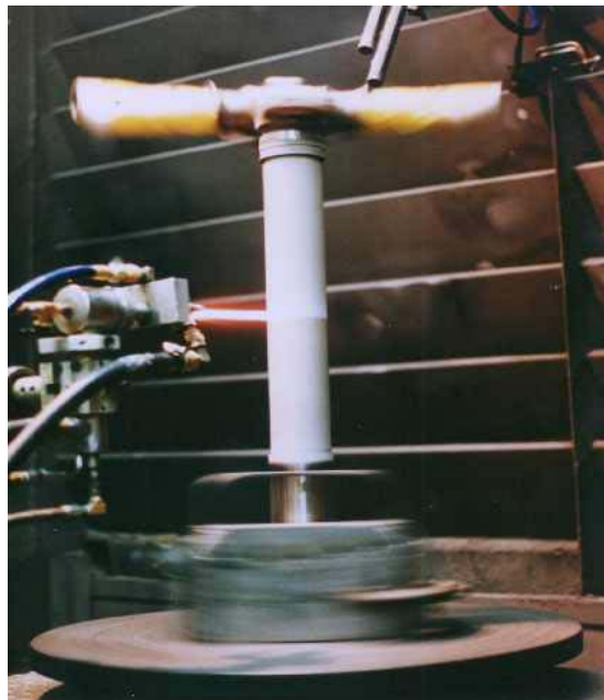
Figure 2. HVOF Spray of Landing Gear Inner Cylinder.
