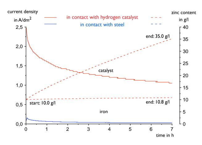
in contact with the SurTec catalyst, zinc dissolves in the average at  $1.5 \text{ A/dm}^2$  (catalyst surface), the dissolution rate is more than 10x greater than with steel
