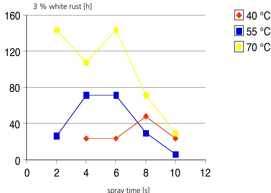
Corrosion protection vs. coating time and temperature for spray application.
