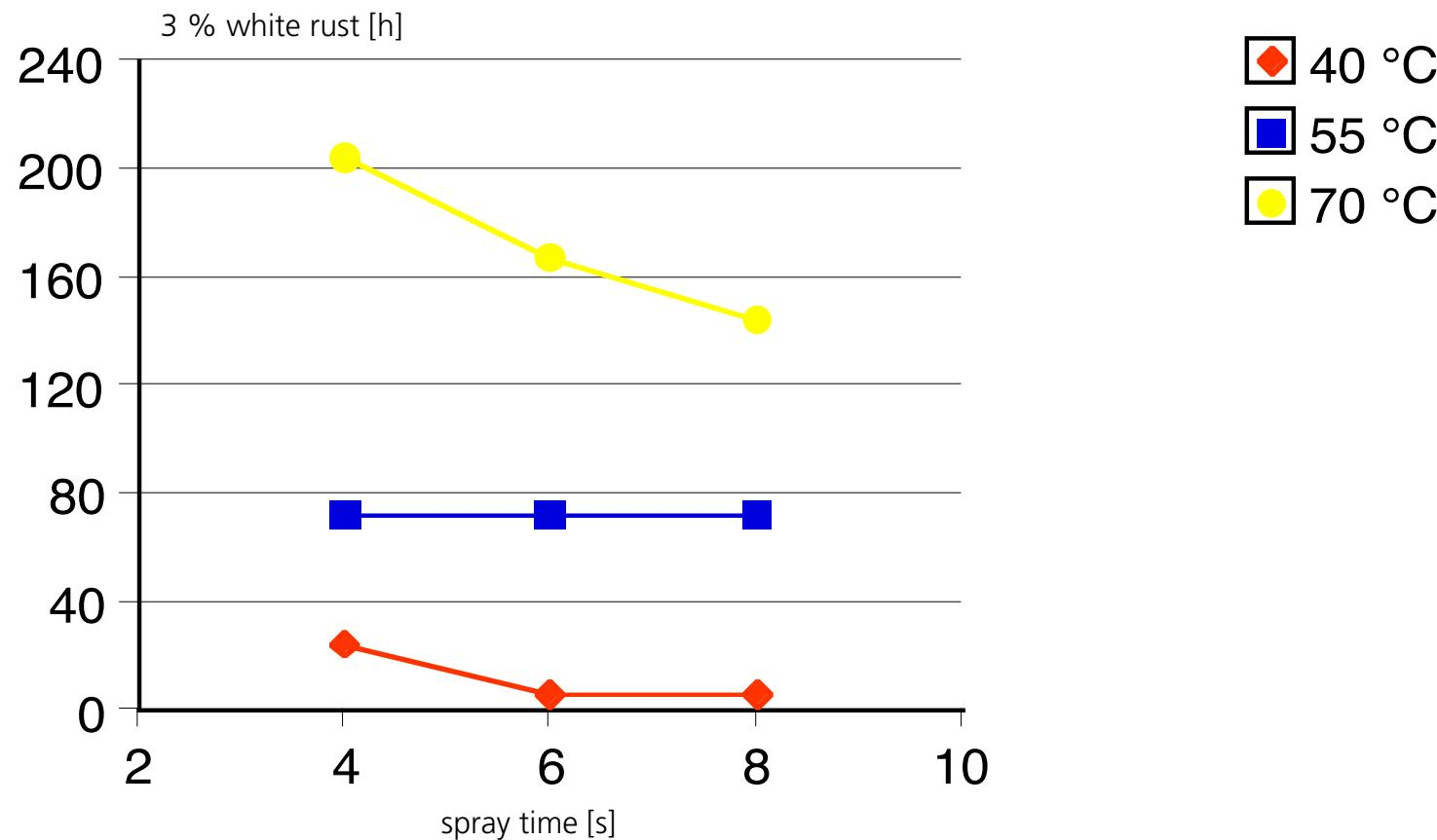
Corrosion protection vs. coating time and temperature for spray application.
