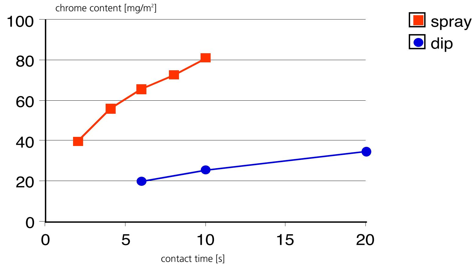
Coating weight of spray and dip application vs. contact time.
