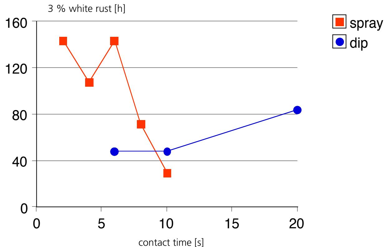
Begin of white rust for spray and dip application vs. contact time.
