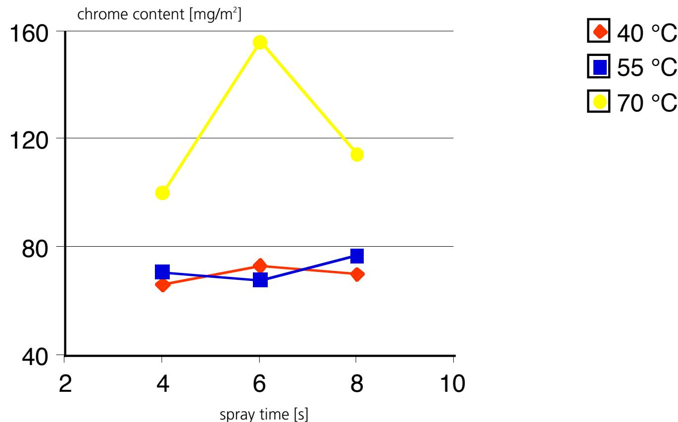
Coating weight vs. coating time and temperature for spray application.
