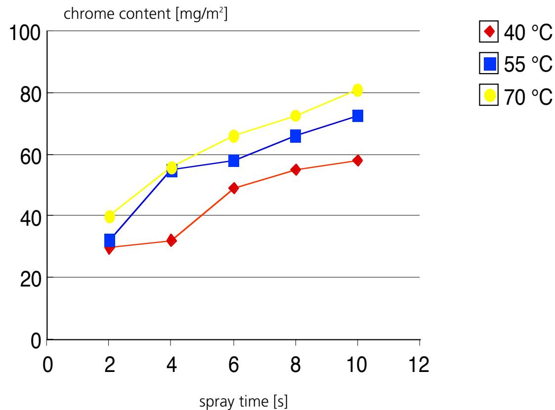
Coating weight vs. coating time and temperature for spray application.
