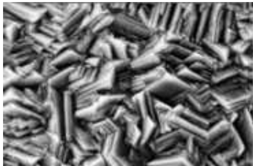
Fig. 8a: Zinc coating with oblique crystals
