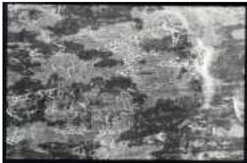
Fig. 6a: CR-sample after pickling without inhibitor and electrolyte contact
