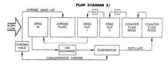
The chrome is then concentrated to 35-37 oz. per gallon. The concentrated chrome is held in a vessel and an automatic feed system transfers the solution to the plating tanks on demand.
