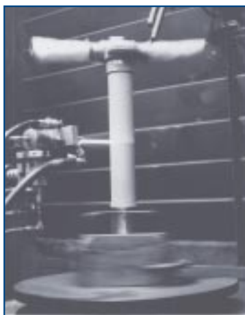
Figure 1: HVOF thermal spraying of WC/Co onto a nose landing gear cylinder from a Boeing 737. The cylinder is approximately 0.6 m long.
