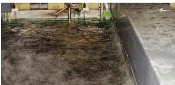
Agitation by pumped flow eductors
