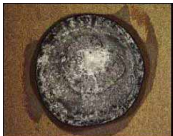
Fig. 19: Printed / wetted area 1000µm / 1760µm (diameter)
