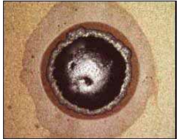
Fig. 17: Printed / wetted area 1000µm / 1100µm (diameter)
