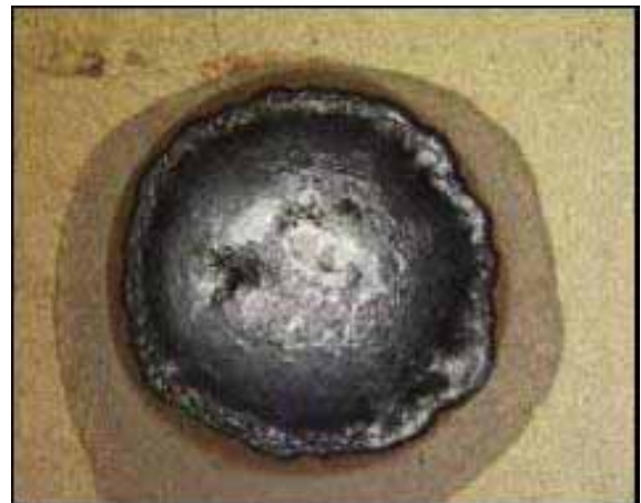
Fig. 18: Printed / wetted area 1000µm / 1400µm (diameter)
