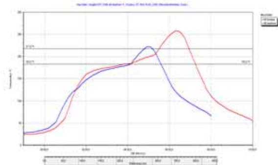
Fig. 16: Reflow profile according to J-STD-020-C (red) in comparison to historical eutectic tin-lead reflow profile (blue)
