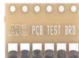
Image 1: Standardized test vehicle for Metronelec wetting balance.
