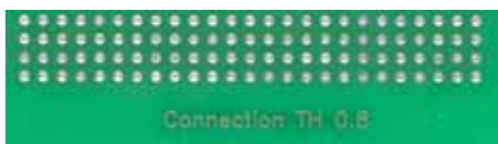
Image 3: 1.00 µm Tin layer after annealing with 2 reflows show complete filling of all 0.8 mm diameter holes.
