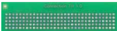
Image 4: 1.00 µm Tin layer after annealing with 2 reflows show complete filling of all 1.0 mm diameter holes.
