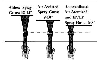
To minimize uneven paint coverage, the operator should hold the gun as perpendicular to the workpiece as possible.
